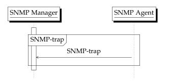
Figure 2.4: SNMP-trap communication
