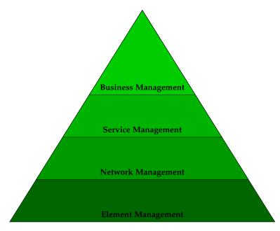
Figure 4.1: Logical layers of the TMN-Model
