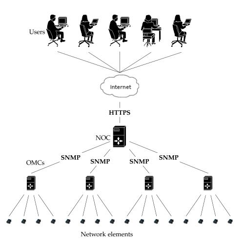
Figure 5.1: Monitor hierarchy of the NOC prototype.
